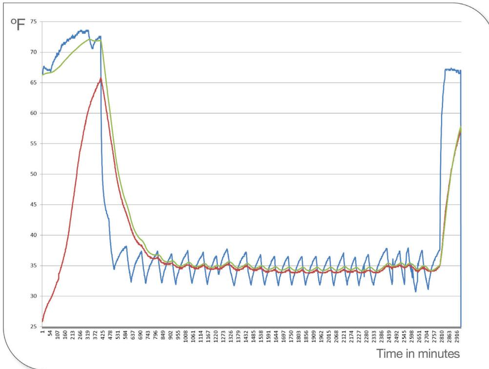
This graph demonstrates the accuracy of product temperature emulation. Actual internal product temperature is measured with a probe, and product emulation is calculated using a mathematical coefficient applied to ambient air temperature in a refrigerated environment.
